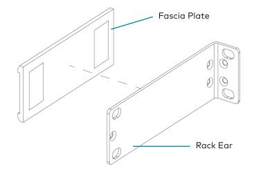
3. Attach the rack ears to the amplifier with the four included  $6-32 \times 3/8$  in. screws.
