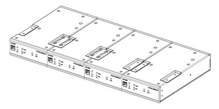
2. Use a Phillips screwdriver (not included) to gang the amplifiers together with three joining plates (two are included with each amplifier) and twelve 8-32 x 5/16 in. screws (four are included with each amplifier).
